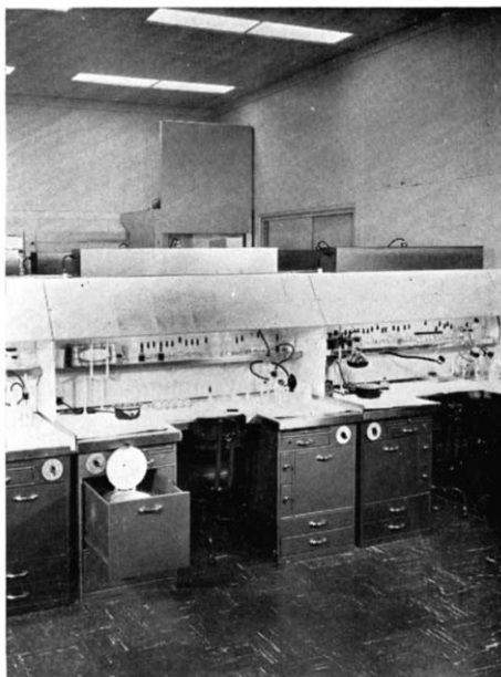
FIG. 15.—Open benches for handling micro-quantities of plutonium.
