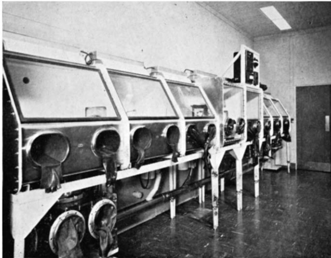
FIG. 4.—Glove box assemblage for work with plutonium-containing solids.
