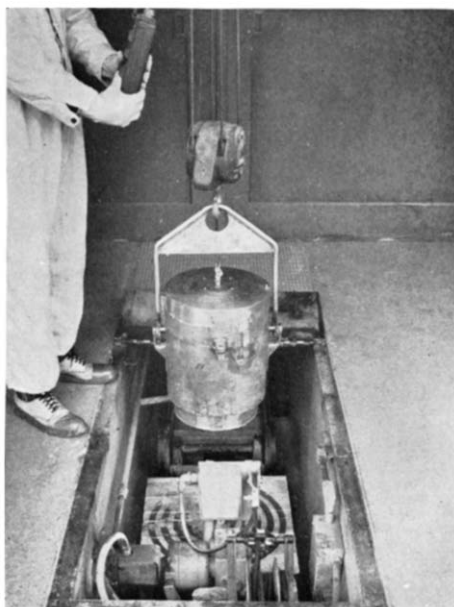
FIG. 2.—Unloading platform and tunnel cart.
