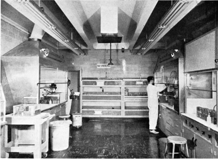
FIG. 24.—Laboratory for receiving, sorting and pretreating samples measuring 1 r/hr at contact.
