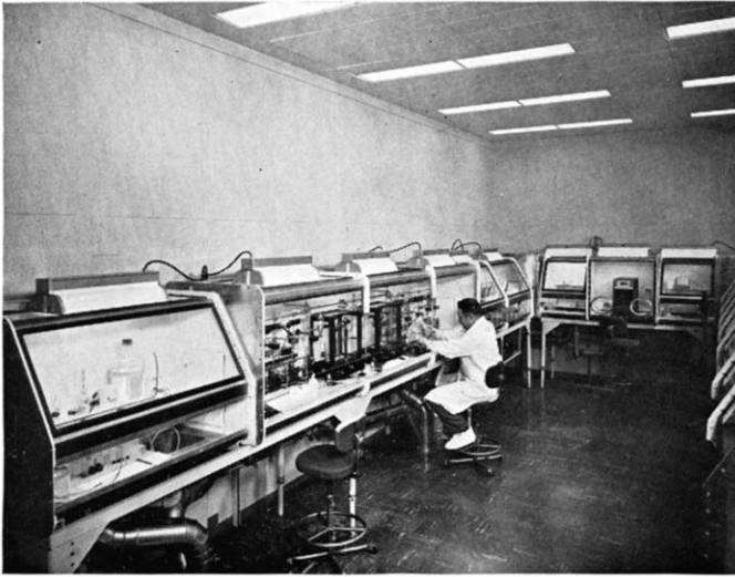
FIG. 1.—Drybox assemblage for assembly line-type of operation.
