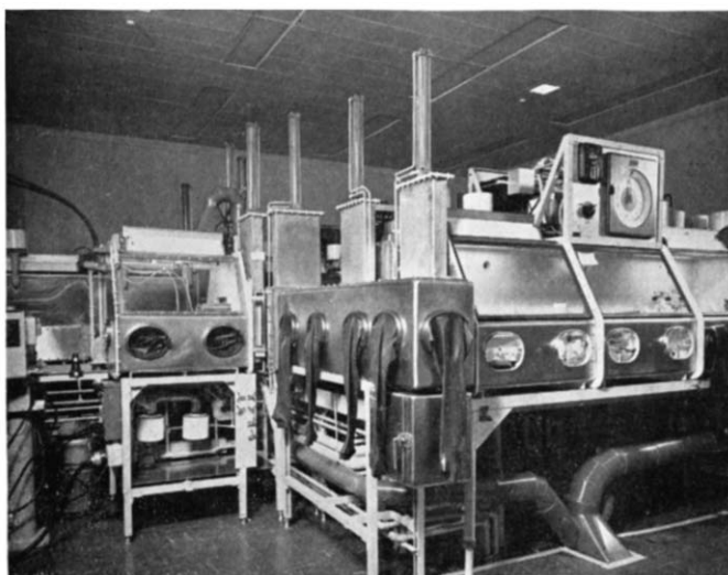
FIG. 16.—Assemblage of dryboxes for spectrochemical operations.
